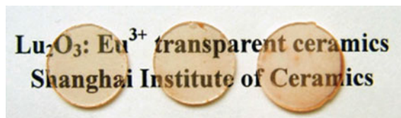
Fig. 2.9 Representative photographs of mirror-polished 5 % \text{Eu}^{3+} -doped \text{Lu}_2\text{O}_3 ceramics sintered at 1850 °C for 6 h, with thickness of 1 mm. Reproduced with permission from [12]. Copyright © 2006, John Wiley & Sons
