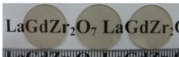
Fig. 2.25 Photographs of the \text{LaGdZr}_2\text{O}_7 ceramics vacuum sintered at 1850 °C for 6 h and annealed at 1500 °C for 5 h in air, with a thickness of 1 mm. Reproduced with permission from [267]. Copyright © 2013, Elsevier
