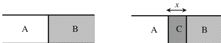
Fig. 3.2 Schematic of solid-state reaction between two single crystals ( A and B ). Reproduced with permission from [47]. Copyright © 2007, Springer
