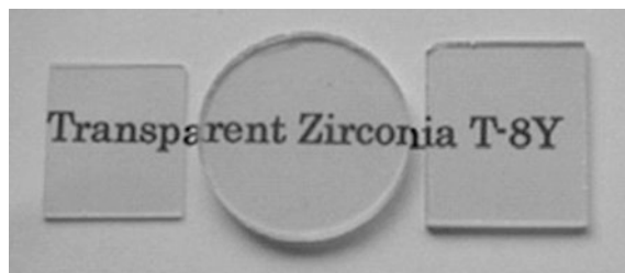
Fig. 2.3 Photographs of representative YZS transparent ceramics, which were made from commercial powder with hot isostatic pressing sintering method. Reproduced with permission from [88]. Copyright © 2008, John Wiley & Sons
